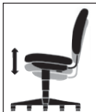
Pneumatic seat height adjustment Regulates height of chair relative to floor.
