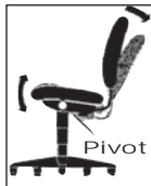
Multi-task control Adjust seat and back angles independently with a single lever (infinite locking within a fixed range).
